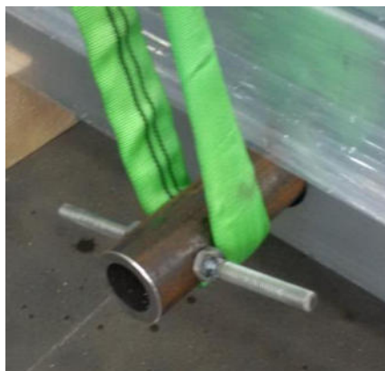
Figure 23: Securing against slippage of the load carrying equipment
