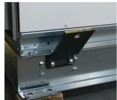
Figure 27: Monobloc crane lifting lugs mounted
