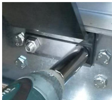
Figure 26: Fixing of the metal sheet and the monobloc crane lifting lug with nuts
