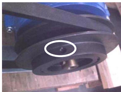
Figure 219: Position of the Allen screws on variable pulleys
