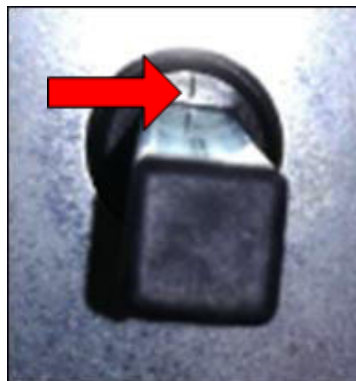
Figure 138: Closed position, characterized by a marking on the gear wheel
