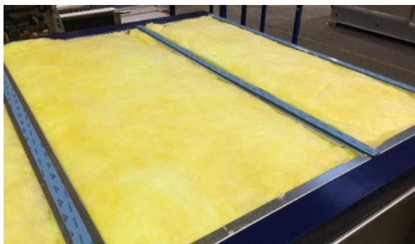
Figure 100: Part of the AHU prepared for assembly of metal sheet roof
