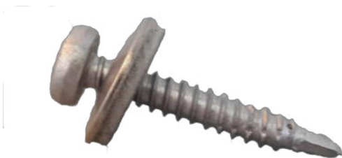
Figure 101: Drilling screw countersunk head TORX 25 with sealing ring ø 4,8 x 30
