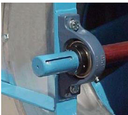
Figure 221: Fan bearing with grease nipple (example Comefri NTHZ)
