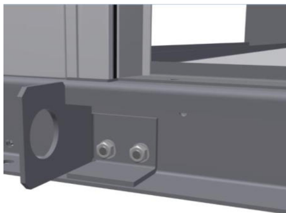
Figure 11: Crane lug mounted
