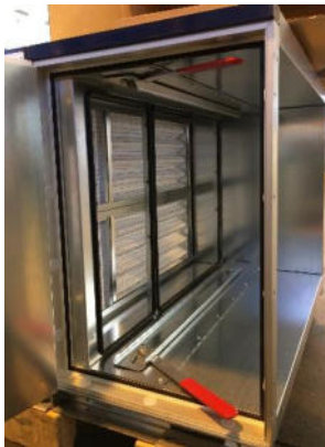
Figure 48: Filter frame for different filter sizes
