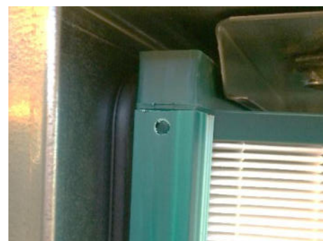
Figure 52: Check, if filter lie on the sealing
