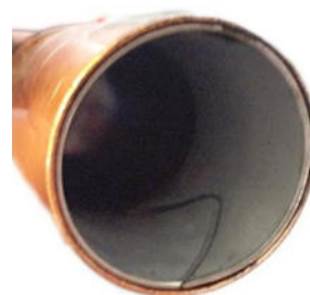
Figure 58: Copper pipe with inserted reinforcing ring
