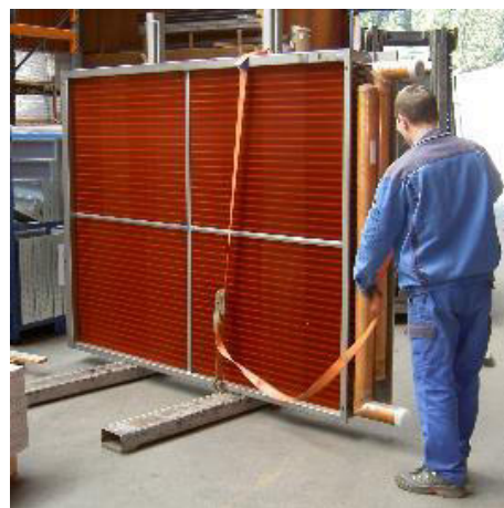
Figure 84: Securing with belt
