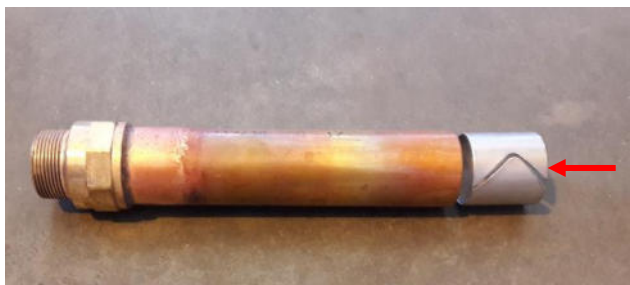
Figure 57: Copper pipe with reinforcing ring
