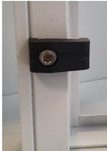
Figure 40: Fixing mechanism at door frame (ZIB)
