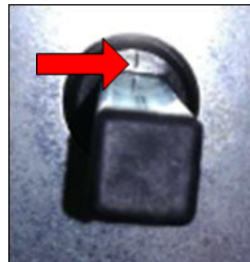
Figure 43: Closed position, characterized by a marking on the gear wheel
