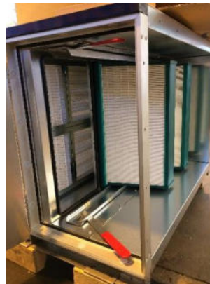
Figure 49: Consider the order according the filter frame raster
