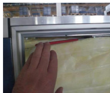
Figure 46: Clamping the filters
