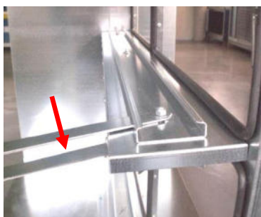
Figure 44: Loosen the clamps
