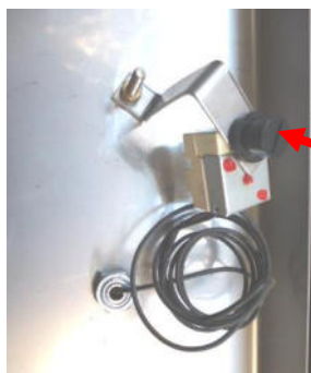
Figure 74: Thermostat with cover cap on the reset button
